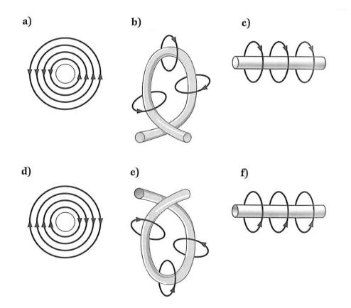
32. For each of the current-carrying solenoids shown below, label the direction that the current is flowing through the solenoid.
