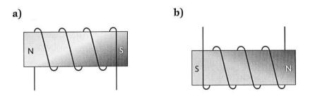
33. For each of the current carrying solenoids shown below, sketch the magnetic field lines around the solenoid. Label which end of the solenoid acts like a north magnetic pole and which end acts like a south magnetic pole.
